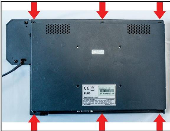
2. Carefully turn the Touch over and gently lift the bottom edge. Lift slowly—there is a cable that you will need to avoid putting any stress on. While holding the cover upright, unplug the black and white cable by lifting the black connector.
