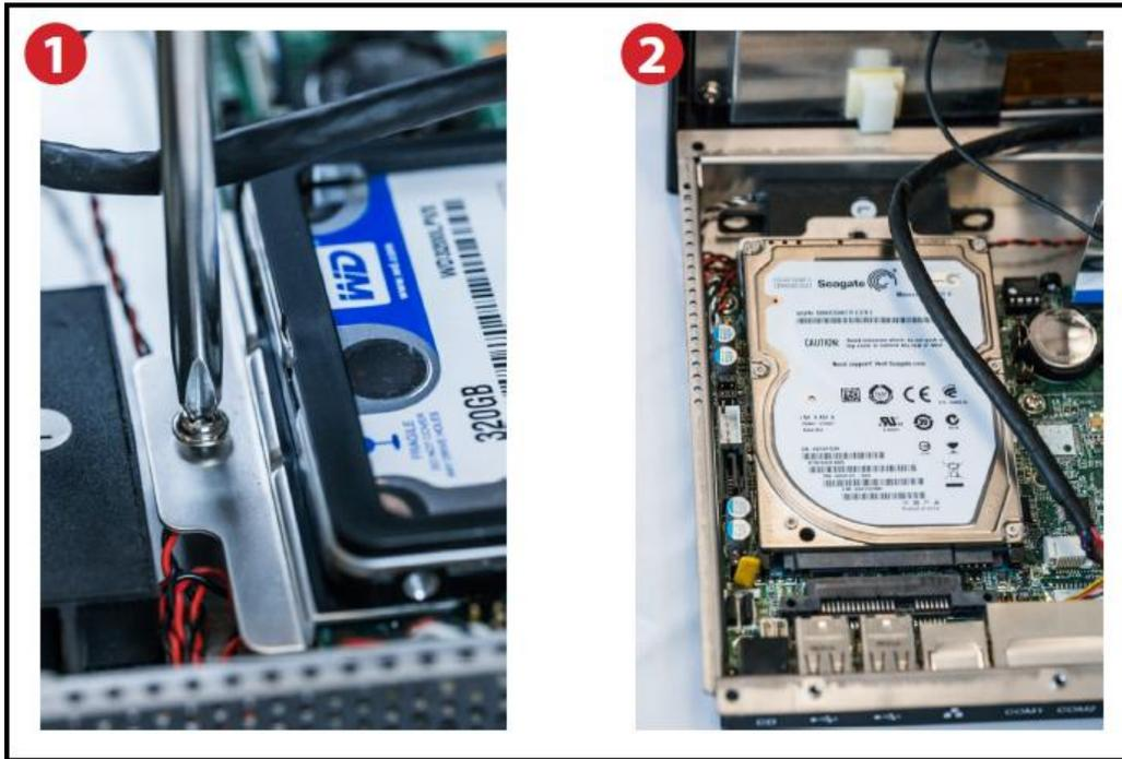
2. Now remove the hard drive mount from the old hard drive. There are two screws underneath the vibration damping pad. Simply roll the pad back and remove both screws. Attach the mount to the new hard drive.
