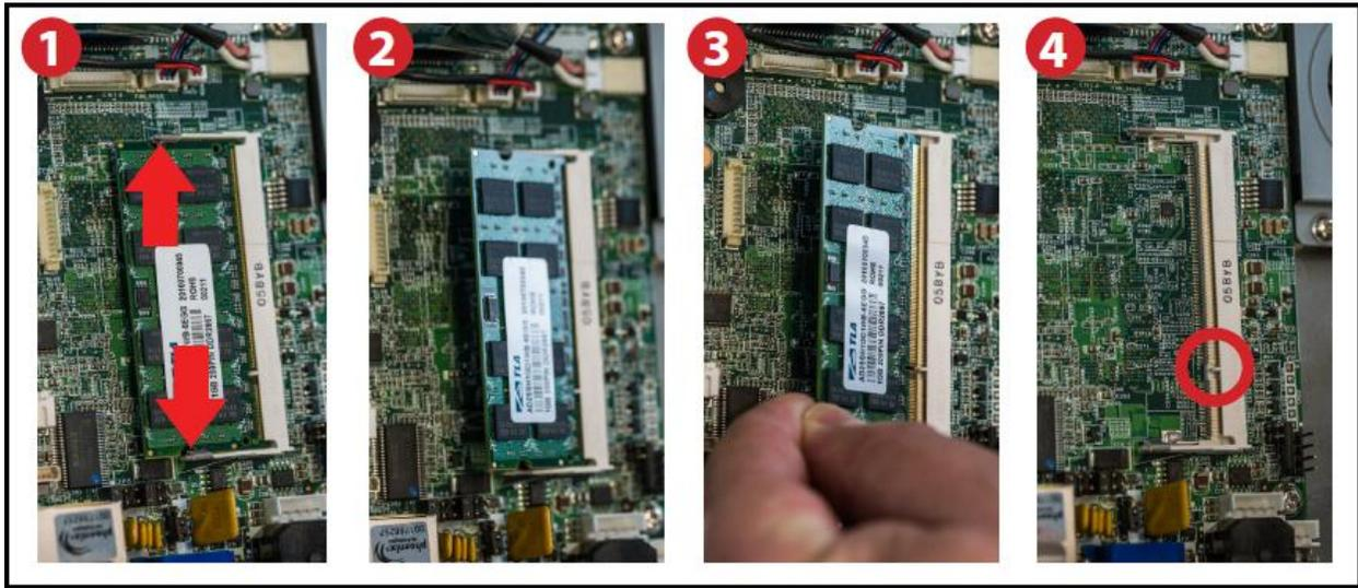
4. Take the new memory chip and align the groove (1) with the notch in the chip slot. Push the chip gently (2) and press the chip down until the tabs snap into place. The chip will be lying flat (3).
