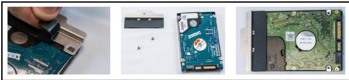
3. Re-insert the drive into the hard drive slot and replace the retaining screw.
