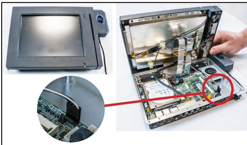
3. Gently spread the clip tabs (1) to release the memory chip. It will pop up on its own (2). Pull the chip to remove it from the slot (3). Note the small notch in the chip slot—the new chip has a groove to match it.
